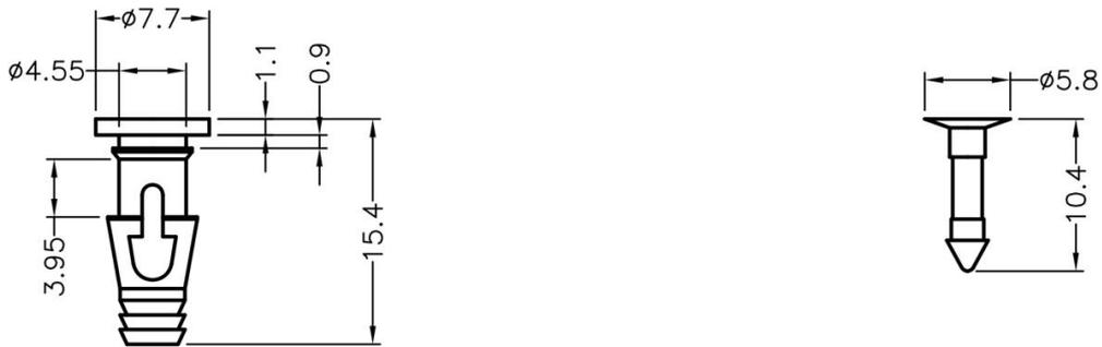
CHASSIS HOLE  $\phi 4.5 \sim 4.7$ mm
