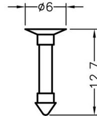
CHASSIS HOLE  $\phi 4.8 \sim \phi 5.0$
