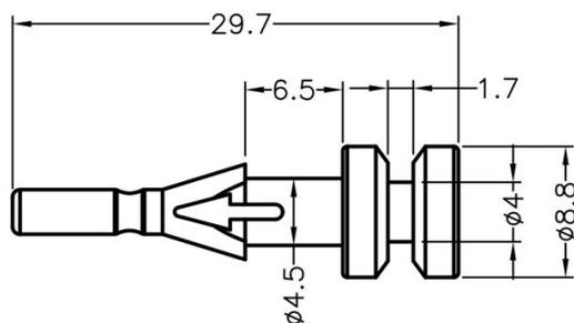
FAN MOUNTING  $\phi 4.5$  THICKNESS 6.8
