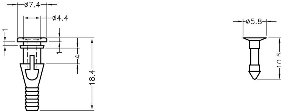
CHASSIS HOLE  $\phi 4.8 \sim \phi 5.0$
